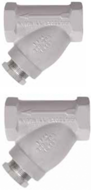
Strainer 1 1/2" F.NPT LPG / NH3 40 Mesh
