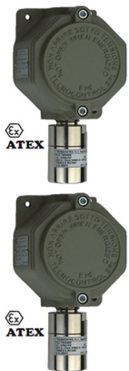
TS293KG ATEX 4-20mA LPG Sensor
